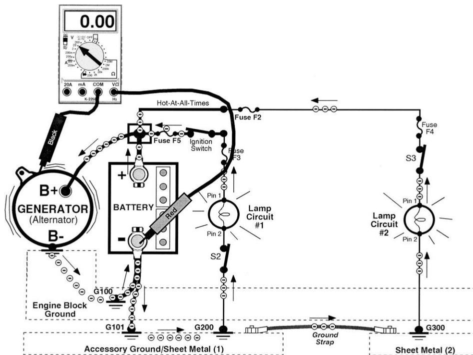
**Proving Both Grounds Are Valid DMM Ground Connections**
